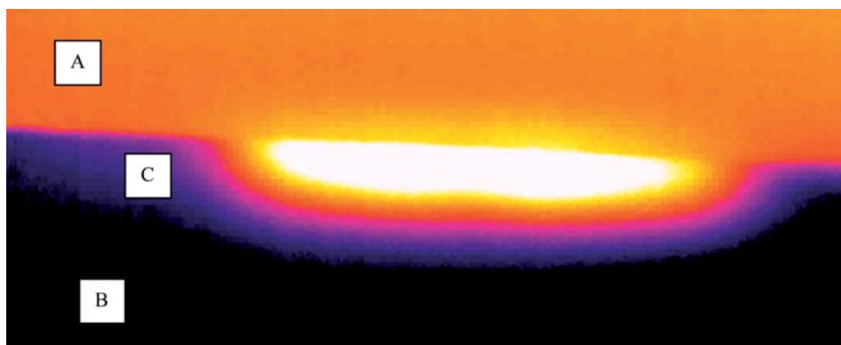
Figure 1. Thermal imaging of the FSR application pulse of EndyMed PRO multi-source RF system (EndyMed Ltd, Caesarea, Israel), showing significant volumetric heating (ThermaCAM SC 640). A – Ambient temperature of air (Orange). B – Ambient temperature of treated medium (Black). C – Varying temperature after FSR pulse.
